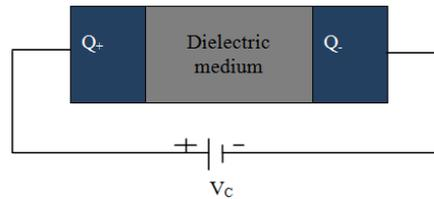
**Figure 12: Parallel Plate Capacitor**
